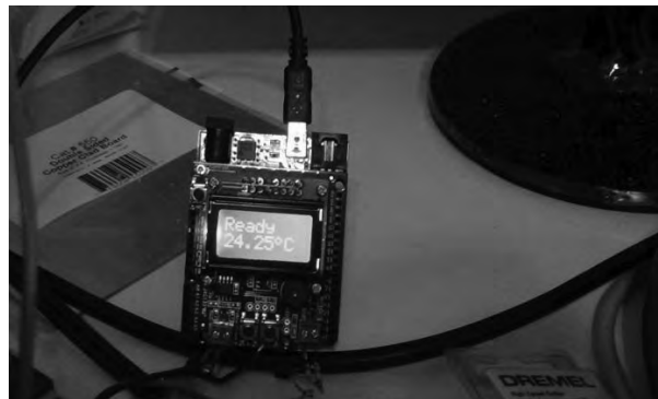
Fig 10. Assembled Oven Controller
