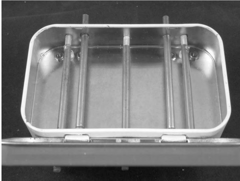
Figure 6 – Interdigital filter with coupled-rod input and side connectors
