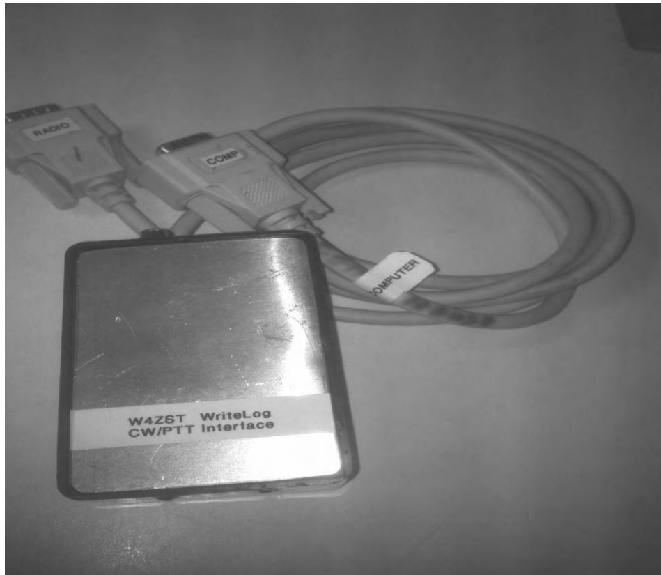
Photo 2: K-3 Interface box. Captive serial cables, LED's, mini phone jacks for PTT and CW. No Audio Isolation
