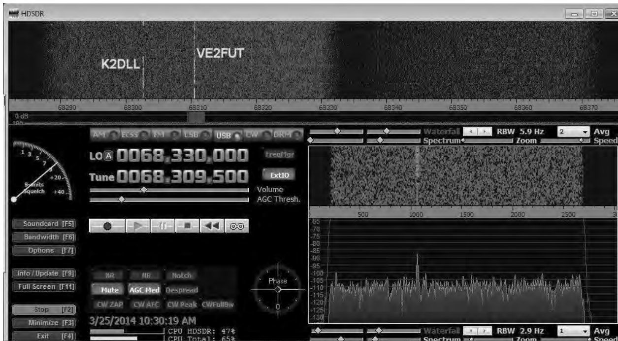
Figure 12 - Preamp after changing L1, receiving two beacons
