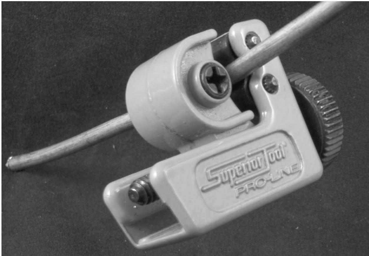
Figure 11 – Preparing semi-rigid coax with miniature tubing cutter
