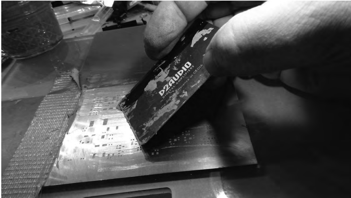
Photo 3. Using an old hotel room key as a squeegee for the solder paste.
