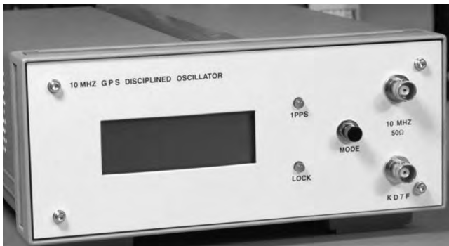
Figure 4. Front panel view of the GPSDO.
