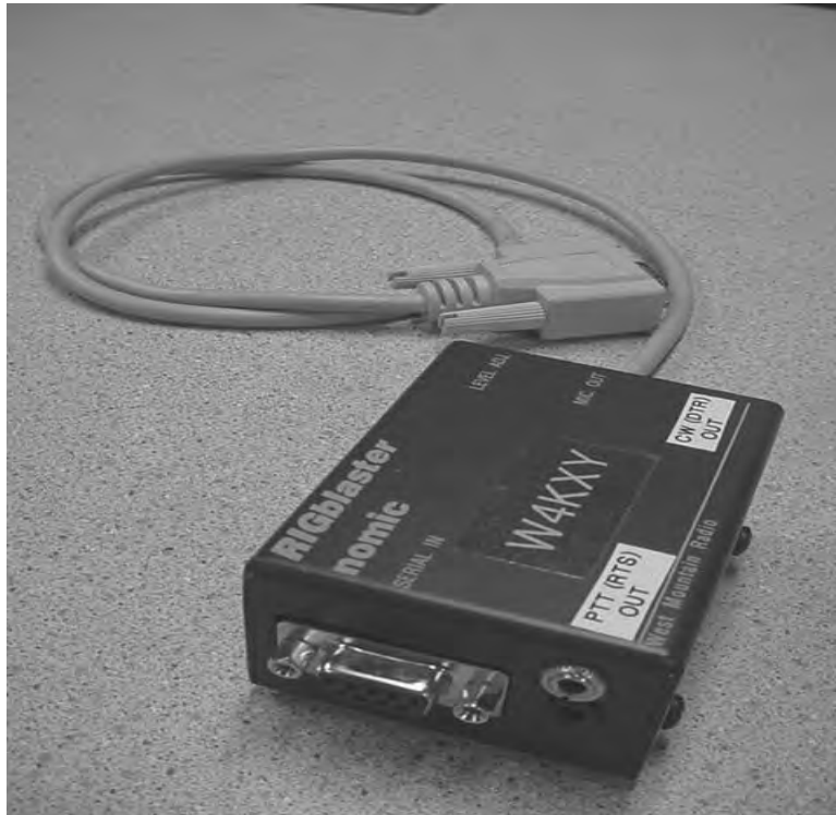
Photo 6: Completed modified RigBlaster Nomic with serial, PTT and CW out
